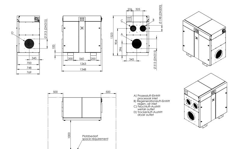
Subject to change without notice. All performance data refer to 1013 mbar, a density of 1.2 kg/m³ and a power supply with 3x400 V/50Hz +PE or 230V/50 Hz. For your project design we recommend to consider a safety discount of 10-20 % for the dehumidification performance depending on the application.
