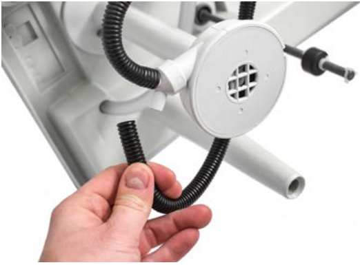
Fig. 7.4.1.5: Pulling off the pump hoses
