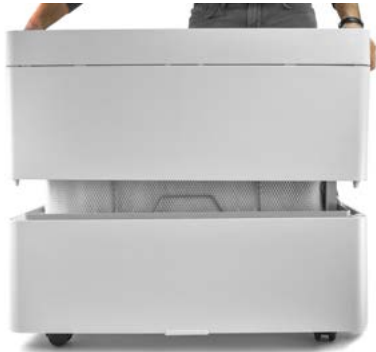
Fig. 6.3.3.1: Removing the upper part of the housing
