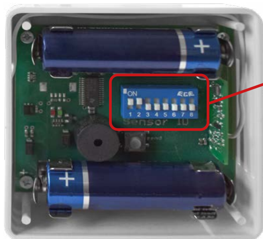
Fig. 5.6.1: Interior view of radio humidity transmitter
