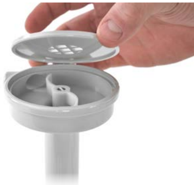
Fig. 6.3.4.9: Fitting the pump cover
