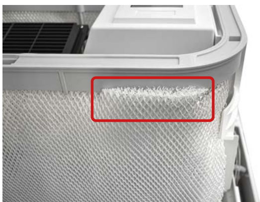
Fig. 6.3.2.5: Incorrect fit of the filter
