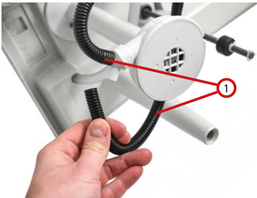
Fig. 6.3.4.4: Pulling off the pump hoses
