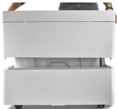
Fig. 6.3.4.2: Removing the upper part of the housing
