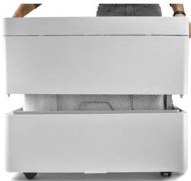
Fig. 6.3.1.1: Removing the upper part of the housing
