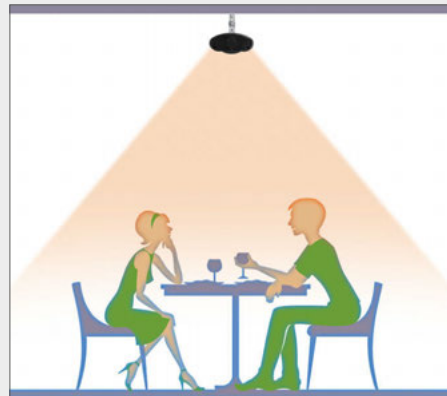
2. The higher the radiator hangs, the wider the heat cone. However, the heat energy is correspondingly lower.
