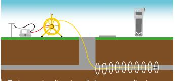
To locate the direction of the non-metalic duct or drain, attach a signal generator to one of the terminals of the Flexitrace and an earth stake (or other independant earth). The Flexitrace can be pushed the length of the duct or drain and then traced along it's complete length with a Cable Avoidance Tool (CAT Receiver).
