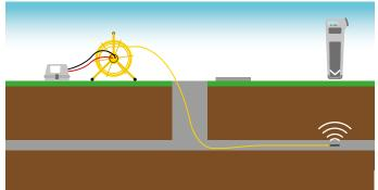
To locate the sonde within a non-metalic duct or drain, you need to energise the end coil, to activate the sonde. This is done by connecting both of the Flexitrace's terminals to the generator. This will allow you to determine the end point and the depth of your duct or drain.
